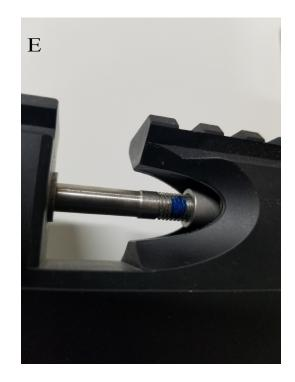
6: Now unscrew the probe from the base as far as you can to get plenty of thread to apply some thread lock to the probe, pictures D & E, now wind the probe in with thread lock on, picture G, and set the tension on the sidelever, you need a good firm closing pressure which should start similar to picture H, too loose and the air will blow when firing, too tight and you will not be able to close the sidelever.
