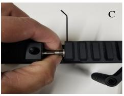
2: Remove the 2 screws located in the side of the bolt body, Picture B, make sure you hold the probe as once they are removed the probe could spring forward, remove the assembly through where the barrel was fitted, Picture C.
